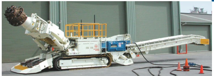
The Mitsui S200MA Roadheader following its refurbishment in Melbourne.
